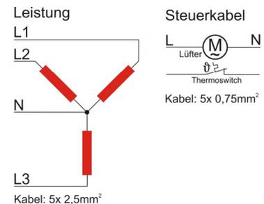
**IRD E380DSM** – 3x 2 kW / 400 V + N + PE (50/60 Hz)
