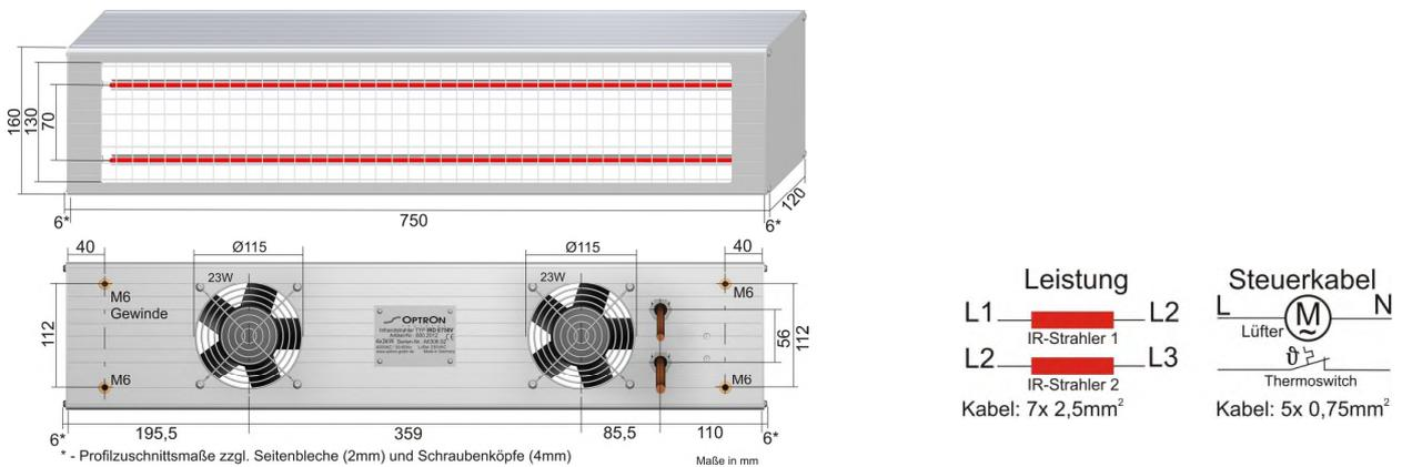
**IRD E750DSM** - 3x 3 kW / 400 V + N + PE (50/60 Hz);
